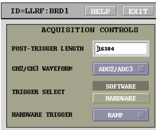
Figure 9: Waveform acquisition configuration panel.
